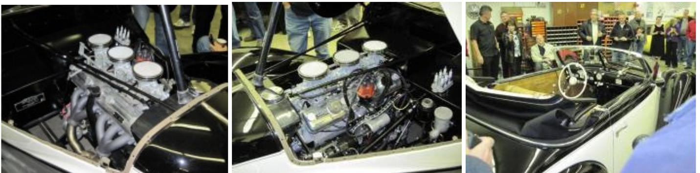
At first glance, the engine appears to have the typical, double overhead camshafts but actually the opposed valves are operated by a single, low-mounted camshaft through a unique combination of multiple push rods and rockers. Various versions of the 327 / 328 won many races and rallies, and the same engine continued to be used very successfully in Frazer-Nash, Bristol and AC cars in the postwar years.
